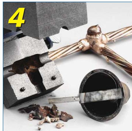
4 Open the mold and remove the expended steel cup – no special disposal required
